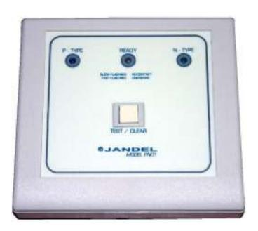
The Jandel Engineering model PN01 **P/N Typing Unit** plugs into a standard Jandel four point probe so that the probe can be used to measure whether a material is P or N type. It is not necessary to use the Jandel four point probe electronics. The probe unit that would normally plug into the Jandel electronics can instead plug into this typing unit to provide a simple system for determining P or N type. It includes an AC adaptor.
